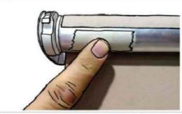
This picture shows how to correct fabric run-off from the left-hand side. Simply stick a small (~3 cm long) strip of masking tape to the aluminium tube
