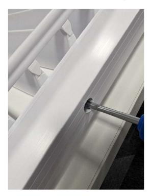
**Note:** Exercise caution to avoid over-tightening as this could potentially damage the louvre and impede its operation.
