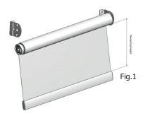
**Note** - the spring end is always on the left hand side and with the fabric rolling from the back of the blind.
