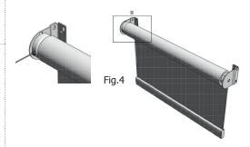
**2.** Gently remove the blind from the brackets and roll back up by hand, then replace it back into the brackets and release the pin (Fig.5) and pull down to the drop (Fig.6), then test to see if the blind returns to the top.
