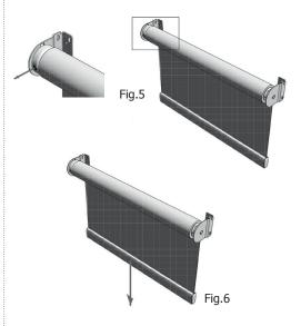
**3.** If not pull the blind and lock off, depress the locking pin and gently remove the blind and roll up by hand. Replace back into the brackets and test again with the locating pin at the front, remembering to release the locking pin before operation.
